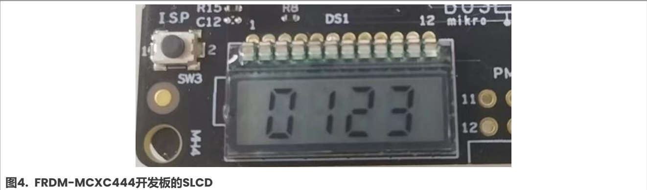
图4. FRDM-MCXC444开发板的SLCD
